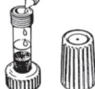
Press the plunger down slowly until it touches the mixture, now place on the cap and screw down slowly until you see the solution filter into the plunger inside.
